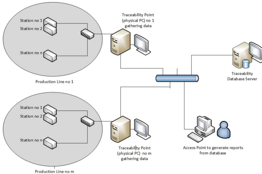
Fig. 6. Distributed hardware architecture of a PFC system [source: own development].
