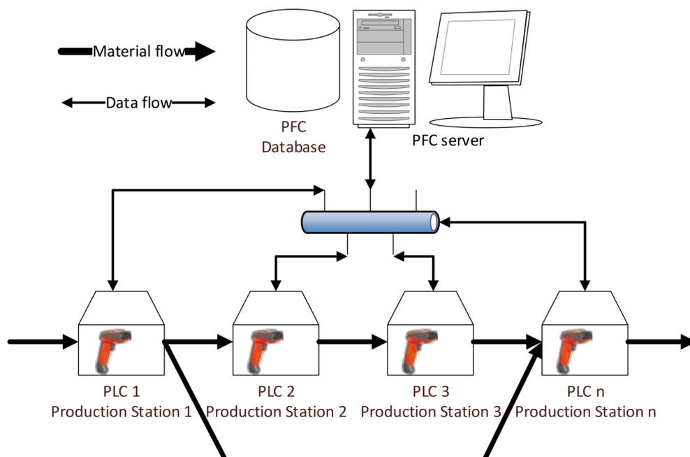
Fig. 1. Principle of PFC system operation with the case of two different material flows/routes [source: own development].
