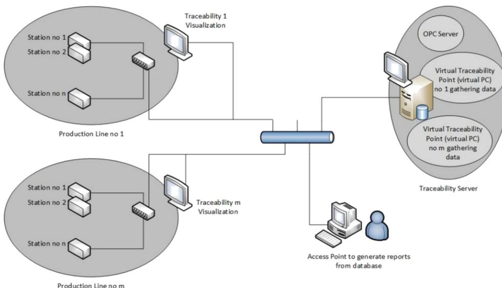
Fig. 7. Central server architecture of a PFC system.
